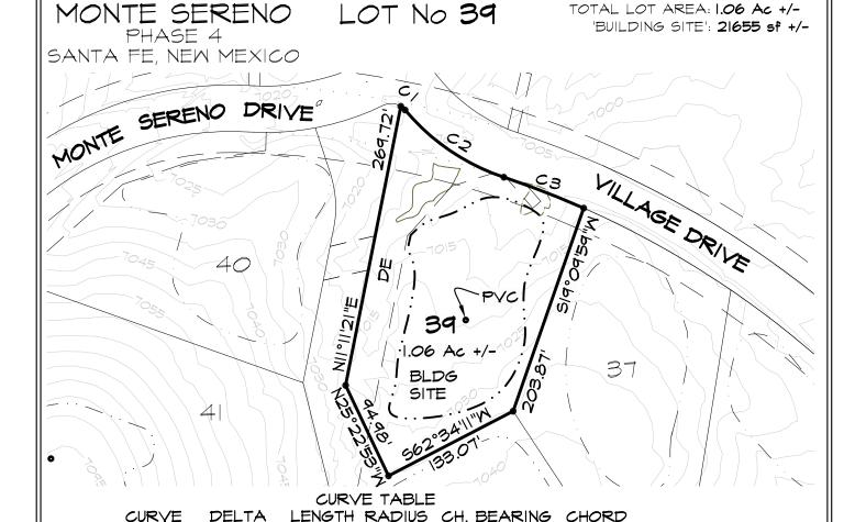
I. DUE TO ROAD CONSTRUCTION, FRONT LOT CORNERS ARE OFFSET 20' FROM THE R.O.W. FRONT LOT CORNERS ARE REFERENCED BY A REBAR SET AT THE INTERSECTION OF SIDE LOT LINES WITH THE 20' OFFSET LINE SHOWN WITHIN THE LOT.
